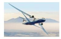
drag is reduced and therefore the engine performance requirements can be reduced. The high wings allow for larger engine sizes, e.g. open rotors.
