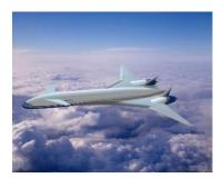
Blended wing: Wide airfoil-shaped bodies and efficient high-lift wings enable significant lift-to-
